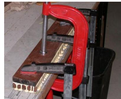
The next step will be the one that's different and makes the "twist" happen. I glued a small strip of wood on one edge of the glued up assembly that is about 3/8 inches square. You can see how that looks in the photos below.
