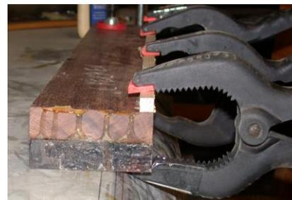
Now that that's in place I'm ready to go to the planer. The idea is that I place the entire assembly into the planer with that strip of wood facing down. This will hold the assembly on an angle so that as I plane it off bit by bit it effectively angles the plane of intersection of the Chechen and Bubinga relative to horizontal. You can see that happening in these photos:
