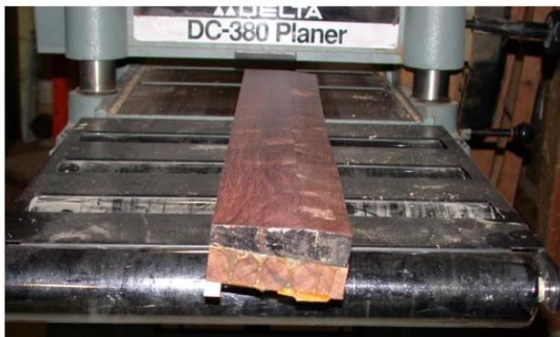
Once you get the first side flat all the way across you just flip it over and plane the other side parallel, and in the process that small strip of wood that kicked up one side will be taken off. Now I'm ready to add the strip of Birdseye Maple to complete the assembly that I'll cut the segments from. Once that's on I trim the sides to the required 22 ½ degrees on the table saw.
